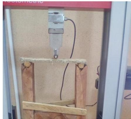
Figure 3. Flexural test showing a sample under a load in a three-point bending setup.
