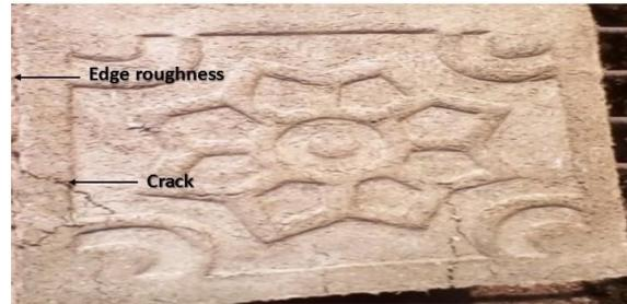
**Figure 5.** First cast (Sample E: 45 – 45 -10 weight %) of the ceiling board.
