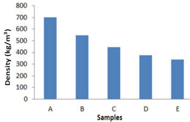
Figure 7. The influence of sample composition on density of the board produced.
