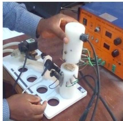
Figure 4. Computer compatible linear heat conduction Apparatus setup for determining thermal conductivity.
