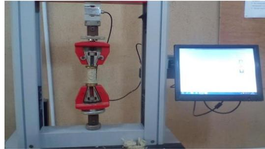
Figure 2. Set up for compressive test.
