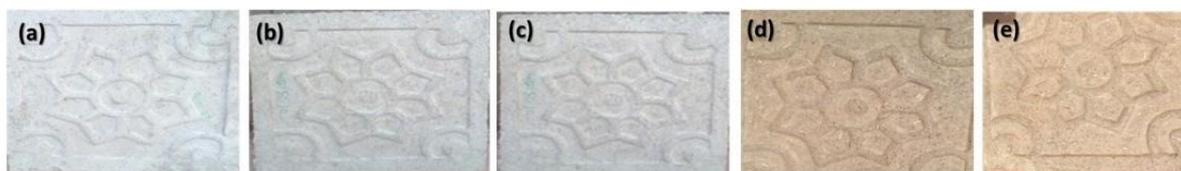
**Figure 6.** Produced ceiling board samples showing color variations.
