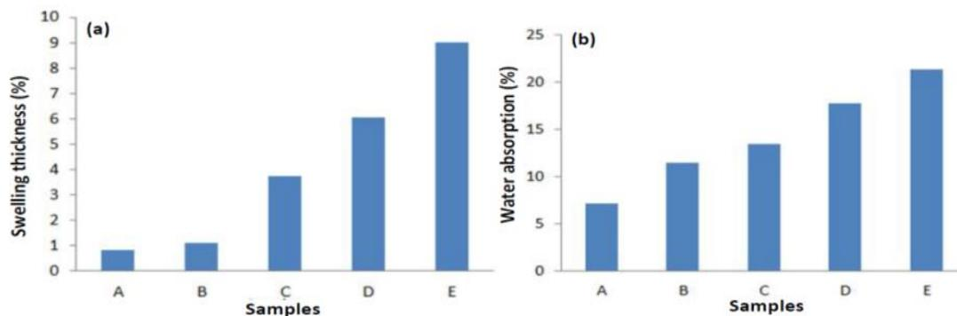
Figure 8. The influence of sample composition on (a) Swelling thickness (b) Water absorption of the ceiling board.
