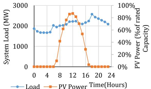
Figure 2. Manah site solar PV system output (clear sky) and recorded MIS system load data on 1 January 2015.
