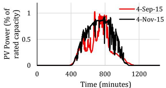
Figure 3. Manah site 1-minute PV power output data for 2 days in 2015 (passing clouds).
