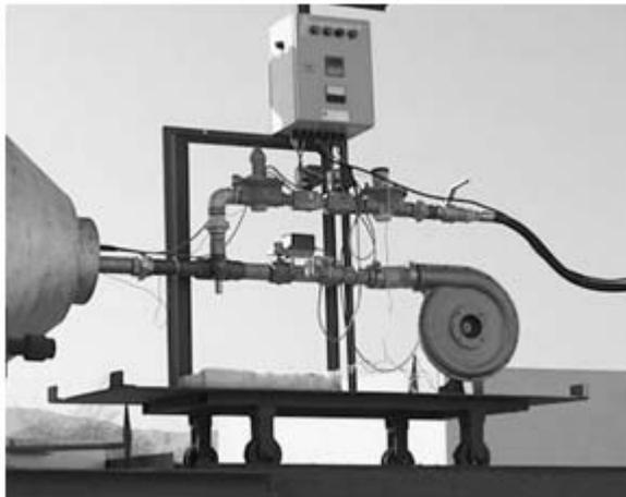
**Figure 9. Burner and blower mounted in the kiln**
