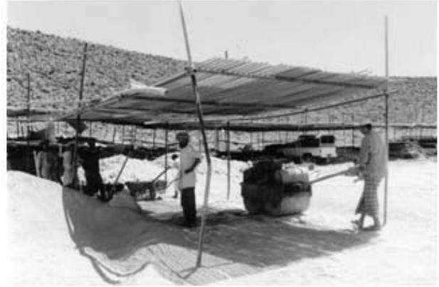
**Figure 3. Grinding of Sarooj**
