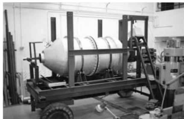
Figure 8. Kiln mounted on a trailer
