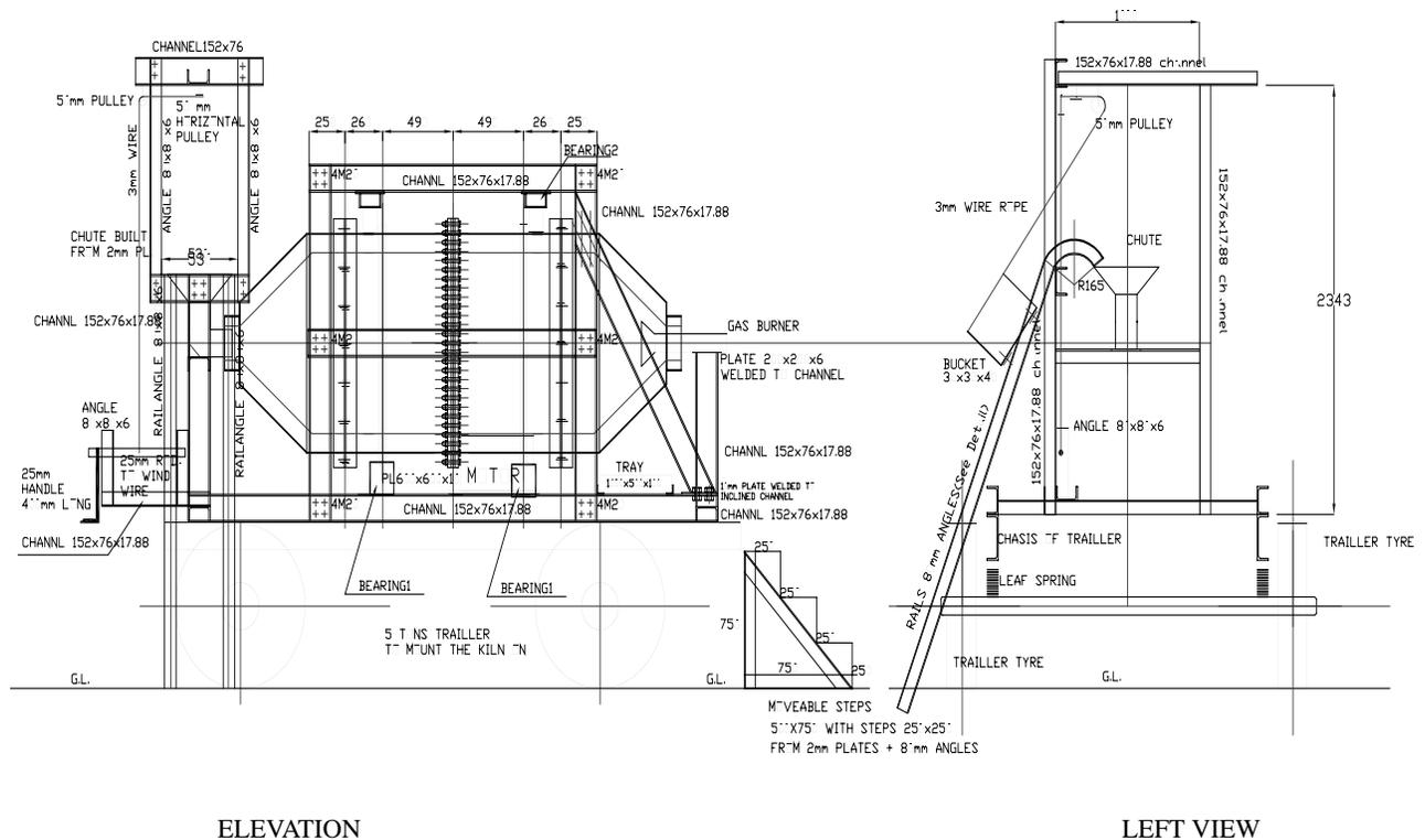
**Figure 10a. Details of the mobile rotary kiln for Sarooj production, Drawing 1/2**
