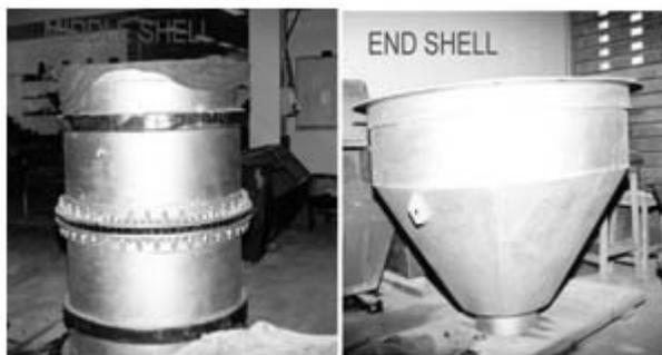
Figure 6. Parts of the rotary kiln
