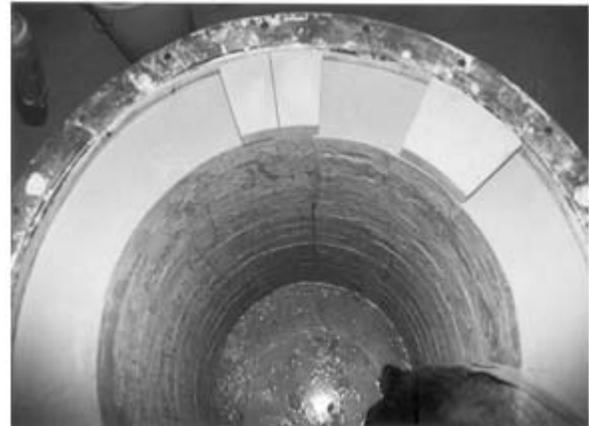
Figure 7. Lining the kiln with fire bricks
