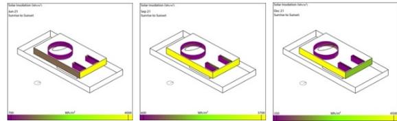
**Figure 14.** Simulation of insolation (in Wh/m<sup>2</sup>) on opaque as well as glazed facades of northwest quadrant for the duration of one day on 21 Jun, 21 Sep, 21 Dec.
