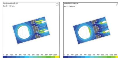
**Figure 18.** Simulation of illuminance levels (Lx) of a typical floor plan on 21 Sep 9 am (left), 3 pm (right).
