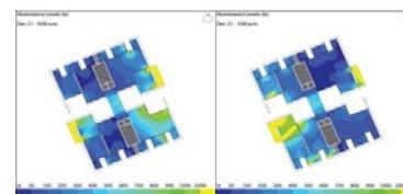
**Figure 13.** Simulation of illuminance levels (lx) of the typical floor plan on 21 Dec 9 am (left), 3 pm (right)
