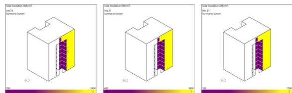
**Figure 7.** Simulation of insolation (in Wh/m<sup>2</sup>) on opaque as well as glazed facades of south-west quadrant for the duration of one day on 21 Jun, 21 Sep, 21 Dec.
