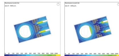
**Figure 17.** Simulation of illuminance levels (Lx) of the typical floor plan on 21 Jun 9 am (left), 3 pm (right).
