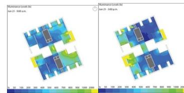
**Figure 11.** Simulation of illuminance levels (lx) of the typical floor plan on 21 Jun 9 am (left), 3 pm (right)
