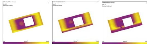
**Figure 15.** Simulation of insolation (in Wh/m<sup>2</sup>) on ground level (garden) for the duration of one day on 21 Jun, 21 Sep, 21 Dec.
