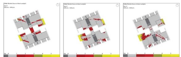
**Figure 10.** Simulation of solar access on typical floor plan between 6 am and 6 pm on 21 Jun, 21 Sep, 21 Dec
