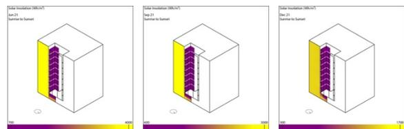
**Figure 8.** Simulation of insolation (in Wh/m<sup>2</sup>) on opaque as well as glazed facades of south-east quadrant for the duration of one day on 21 Jun, 21 Sep, 21 Dec.
