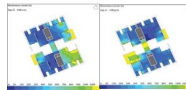
**Figure 12.** Simulation of illuminance levels (lx) of the typical floor plan on 21 Sep 9 am (left), 3 pm (right)
