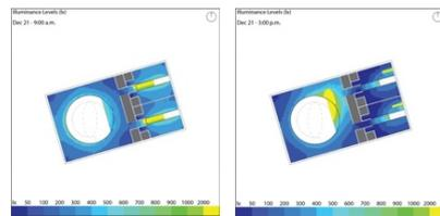
**Figure 19.** Simulation of illuminance levels (Lx) of a typical floor plan on 21 Dec 9 am (left), 3 pm (right).
