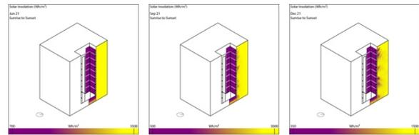
**Figure 9.** Simulation of insolation (in Wh/m<sup>2</sup>) on opaque as well as glazed facades of northeast quadrant for the duration of one day on 21 Jun, 21 Sep, 21 Dec
