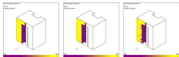
**Figure 6.** Simulation of insolation (in Wh/m<sup>2</sup>) on opaque as well as glazed facades of north-west quadrant for the duration of one day on 21 Jun, 21 Sep, 21 Dec.
