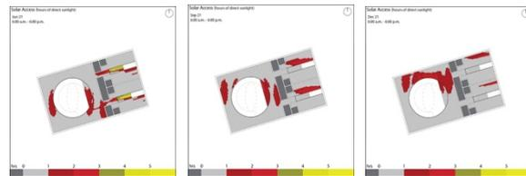
**Figure 16.** Simulation of solar access on typical floor plan between 6 am and 6 pm on 21 Jun, 21 Sep, 21 Dec.
