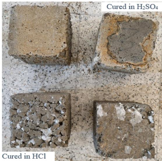
**Figure 9.** The physical condition of concrete specimens after the attack of H<sub>2</sub>SO<sub>4</sub> and HCl.
