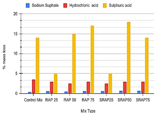
**Figure 10.** Percentage mass loss in mixes after 90 days of sulphate and acid attack
