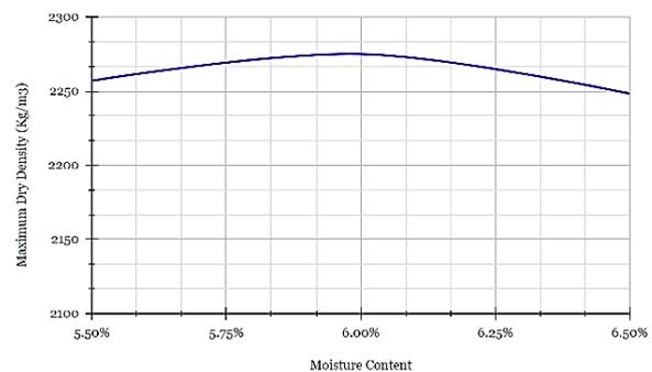
**Figure 2.** The graph between dry density and moisture content
