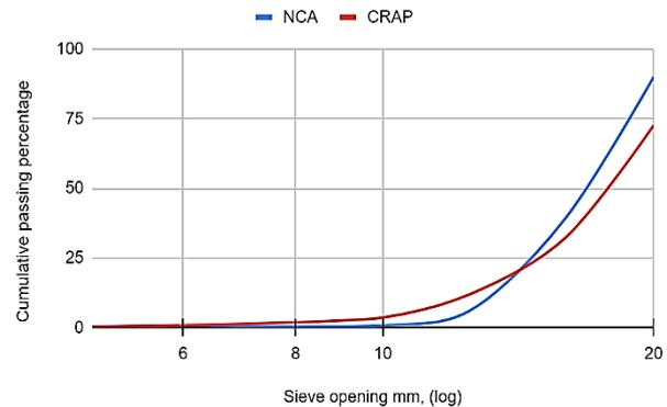
**Figure 1.** Comparison of the particle size distribution of NCA and CRAP.
