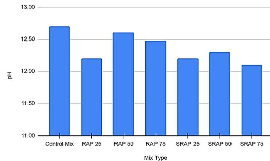
**Figure 8.** Variation of pH in different concrete mixes.
