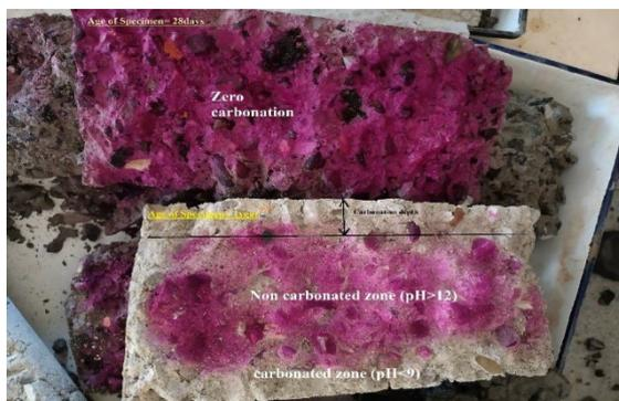
**Figure 7.** Carbonation depth comparison
