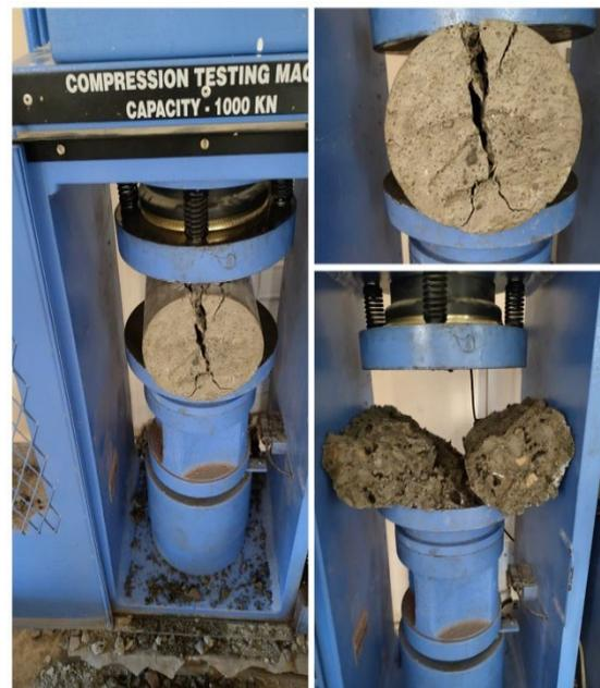
Figure 5. Split tensile strength testing of concrete.
