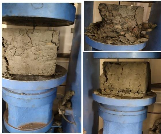
Figure 3. Compression strength testing of concrete
