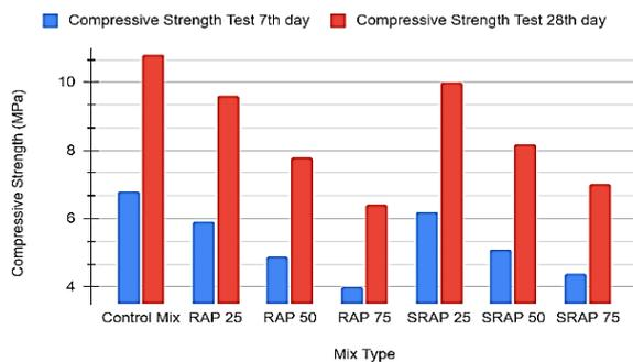
Figure 4. Compressive Strength of DLC on the 7<sup>th</sup> and 28<sup>th</sup> day of curing.
