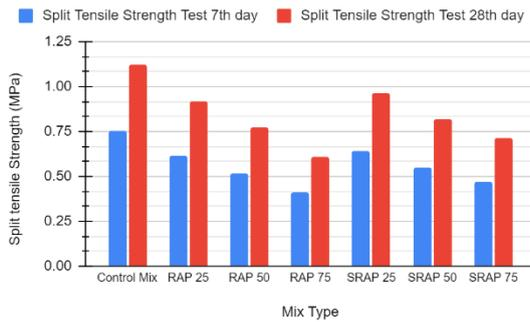
**Figure 6.** Split tensile Strength of DLC on the 7<sup>th</sup> and 28<sup>th</sup> day of curing.
