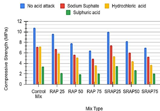
**Figure 11.** Compressive strength of cubes subjected to acid and sulphate attack
