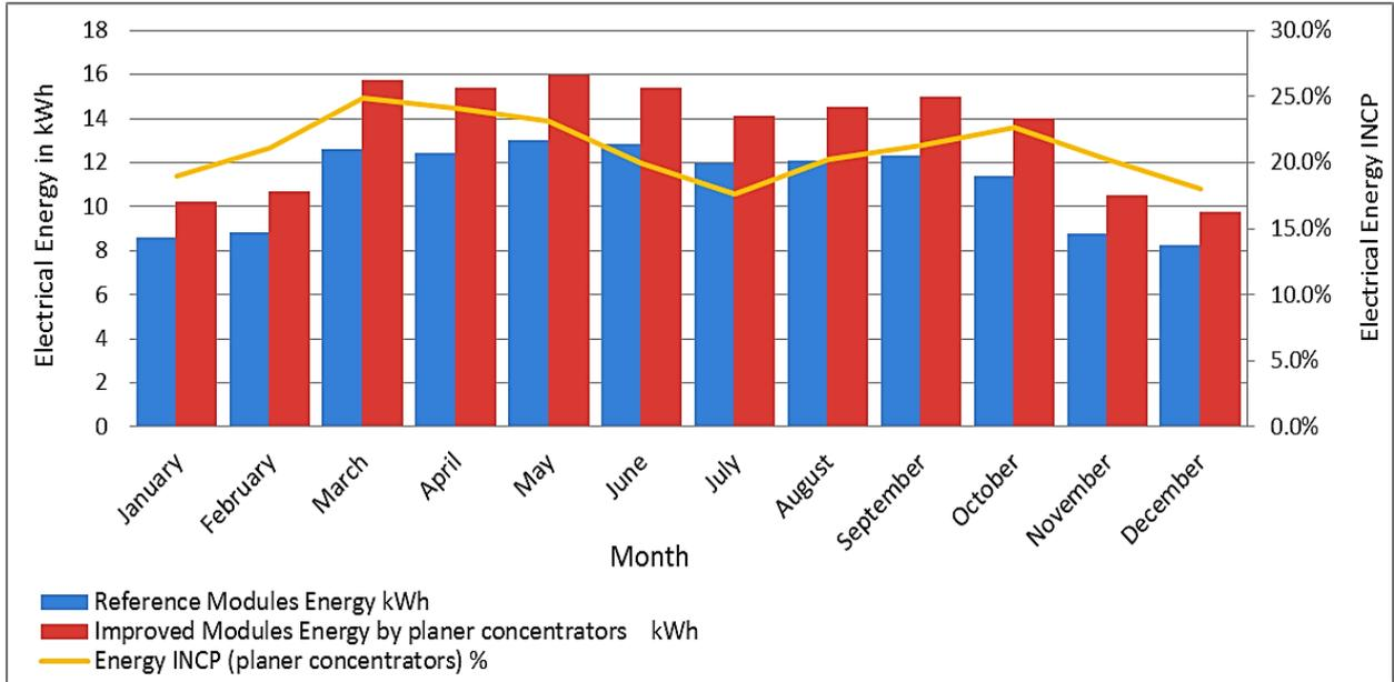
Figure 5. Energy INCP, improved and reference PV modules (groups) energy produced.
