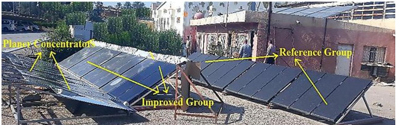
Figure 3. Reference and improved solar PV modules (groups).
