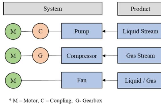
**Figure 1.** General Motor Applications and Setup.
