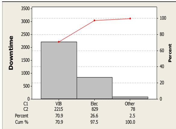
Figure 5. Pareto Chart of Motor Failure Modes.
