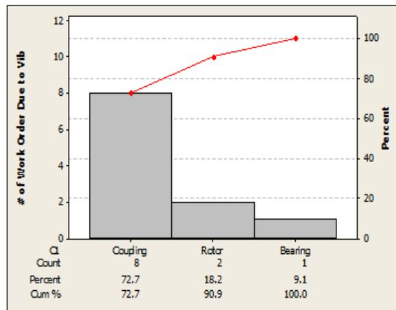
Figure 6. Pareto Chart of Vibration Failures.
