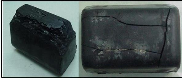
Figure 8. Failure and Cracks of Rubber Blocks.
