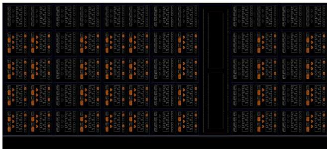
Figure 6. Placement of 128-bit LFSR PUF.
