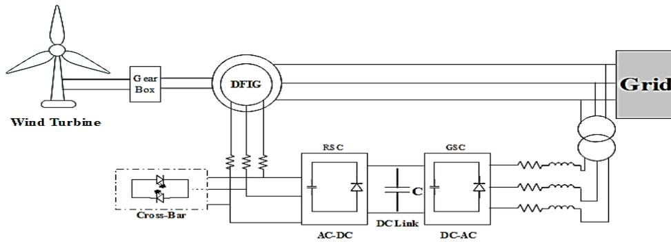
**Figure 1.** Doubly Fed Induction Generator (Yang et al., 2012).
