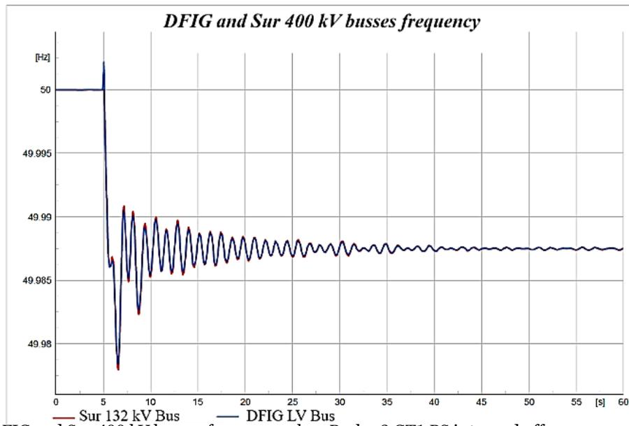
**Figure 13.** DFIG and Sur 400 kV busses frequency when Barka-3 GT1 PS is turned off.
