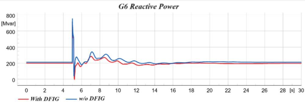
**Figure 4.** Generator 6's active and reactive power without (blue) and with (red) wind farm
