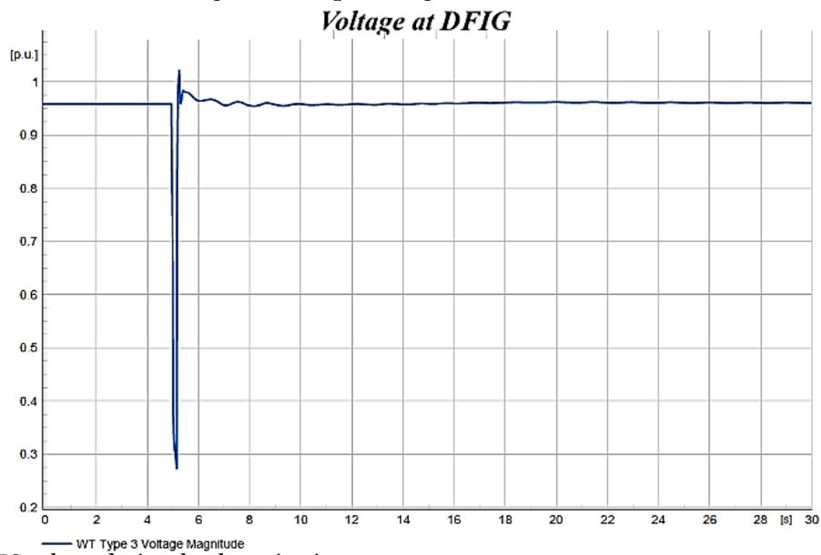
**Figure 7.** DFIG voltage during the short circuit.
