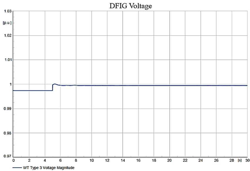
**Figure 15.** DFIG Voltage during load shedding.
