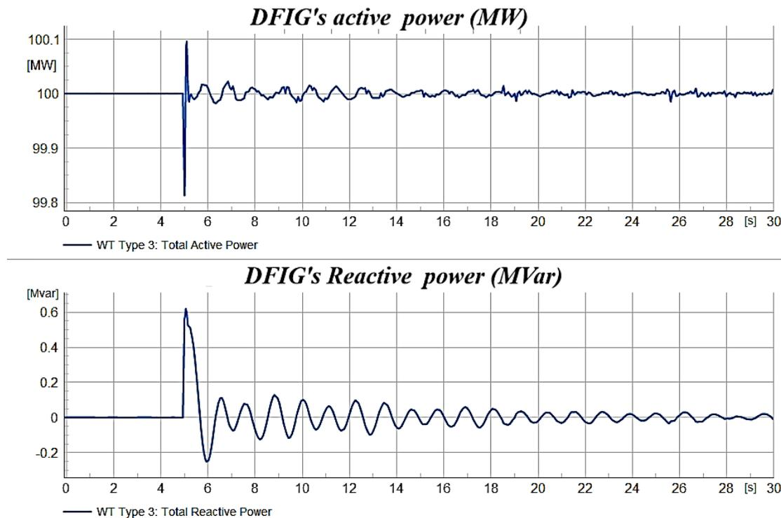
Figure 11. DFIG's active and reactive power while Barka-3 GT1 PS is turned off.
