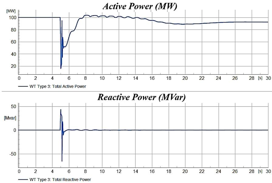
**Figure 6.** DFIG active and reactive power during a three-phase short circuit.
