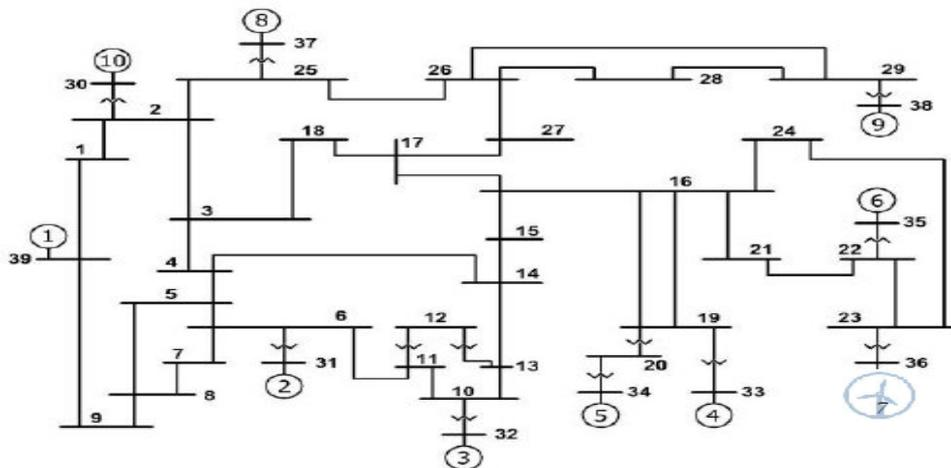
**Figure 2.** Wind farm in a single-line schematic of the IEEE 39-bus, ten machines system.
