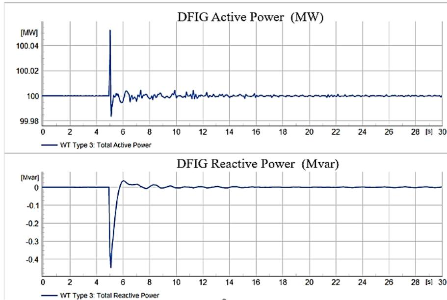
**Figure 14.** DFIG active and reactive power during load shedding.
