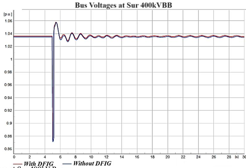
Figure 8. Voltages at Sur 400kV Bus.
