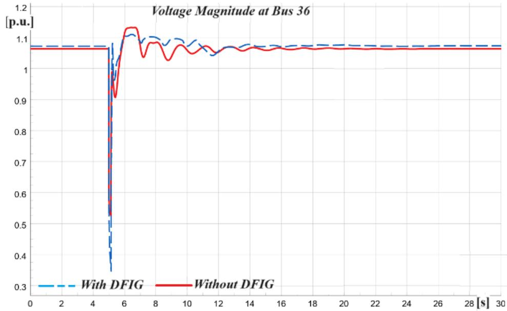
**Figure 3.** The terminal voltage of bus 36 without and with the wind farm
