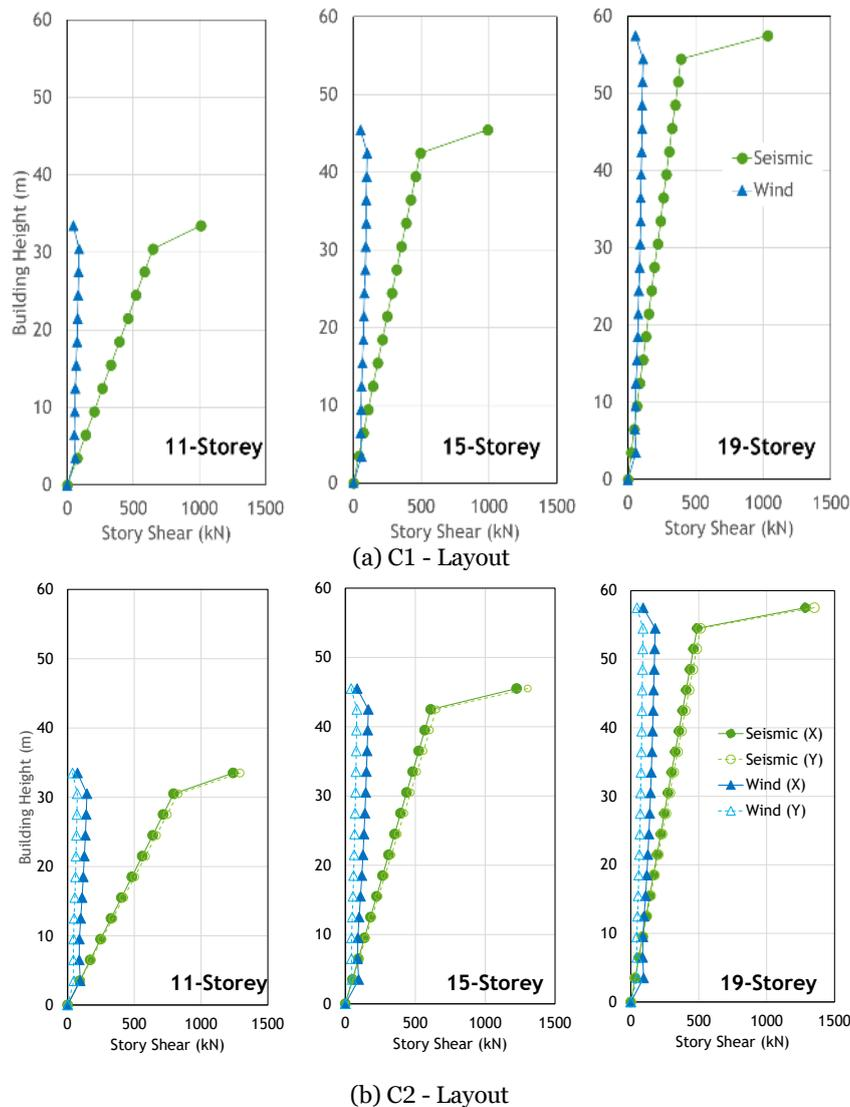
**Figure 5.** Storey Shear Force Distribution - Frame Only (S1)
