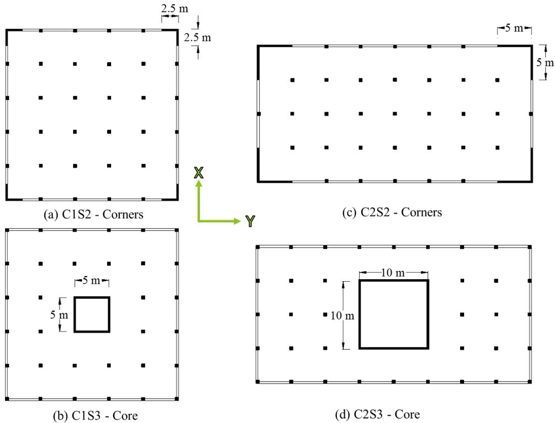
**Figure 2.** Shear wall layout at corners and core in C1 (a & b) and C2 (c & d) aspect ratio
