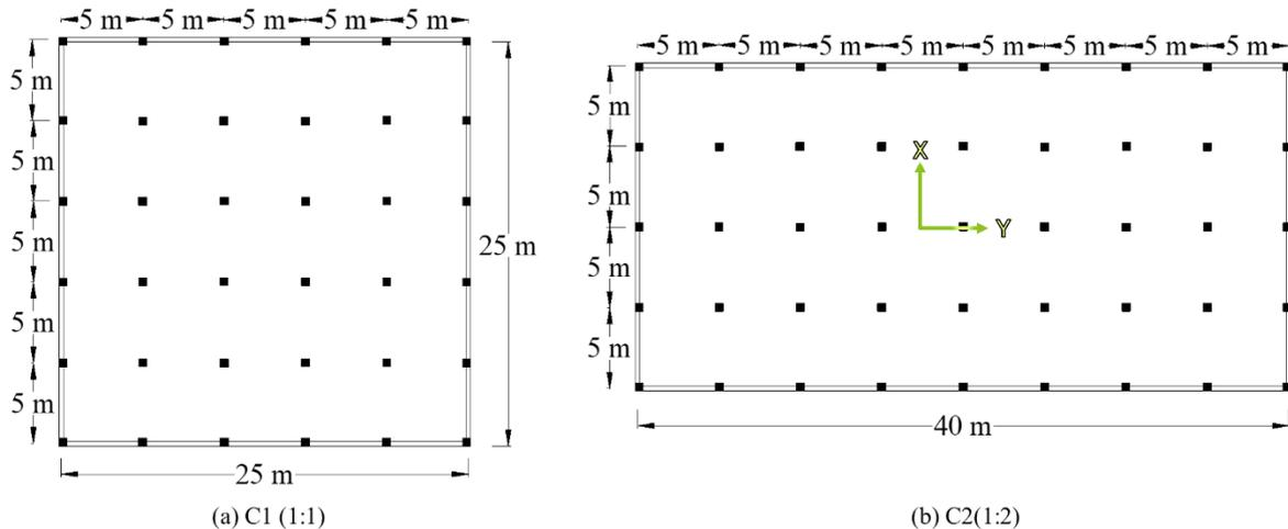
Figure 1. Typical floor plan for the two aspect ratios for all building heights
