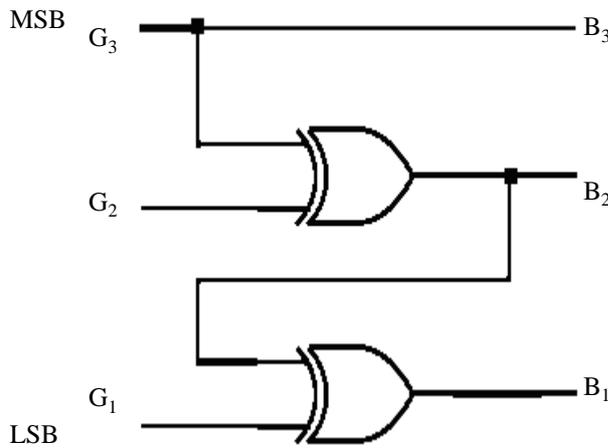
Figure 4. A 3-bit Gray to Binary converter circuit
