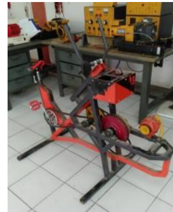
Figure 2. The static bicycle with a car alternator.
