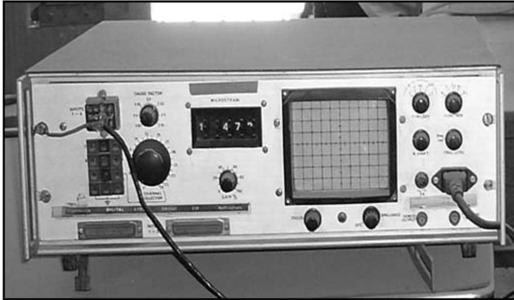
Figure 3. Micro strain meter apparatus used in this study
