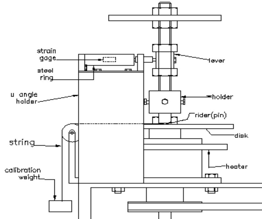
**Figure 2. Four strain gages mounted on steel ring in addition to strain gage calibration system**
