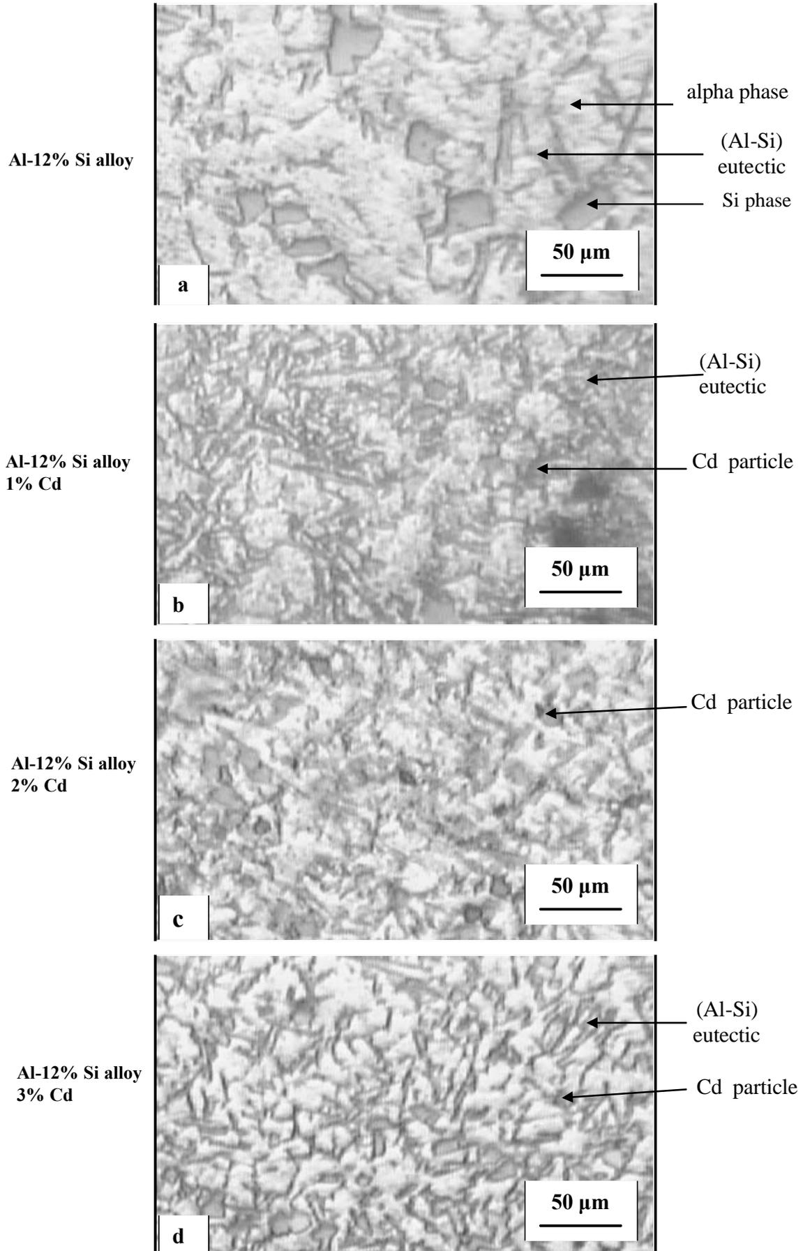
**Figure 5. The microstructures of the studied alloys (as cast)**
