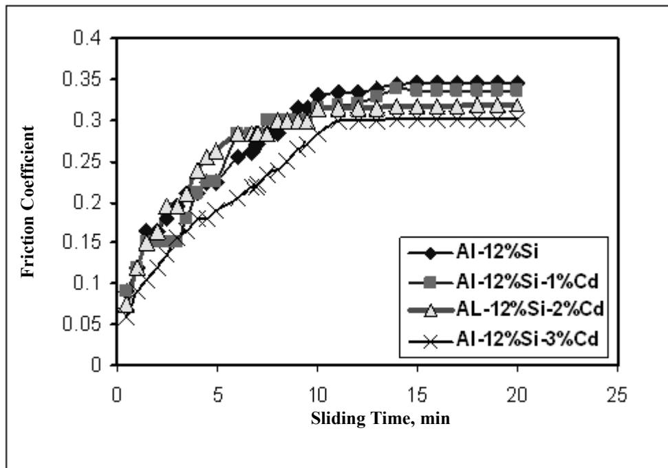
Figure 9. The effect of cadmium adding on friction coefficient ( $\mu$ ) of different alloys at a applied load of 20N and sliding speed of 2.7 m/sec
