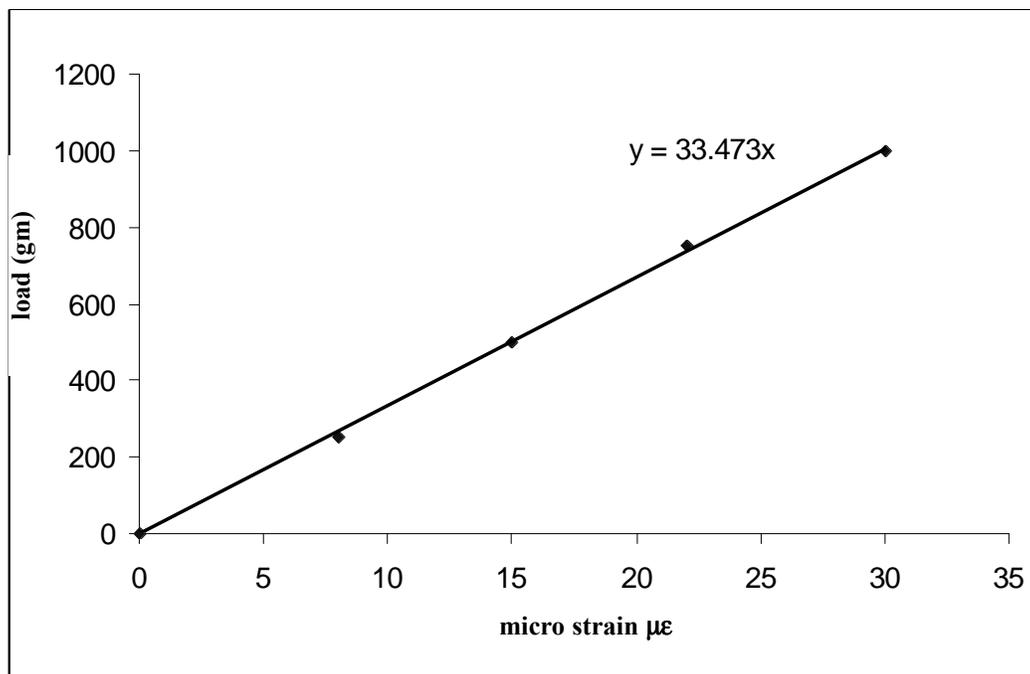
Figure 4. The calibration curve of load versus strain at a constant sliding time of 20 min, sliding speed of 2.7 m/sec. and steel disc hardness of 35 HRC
