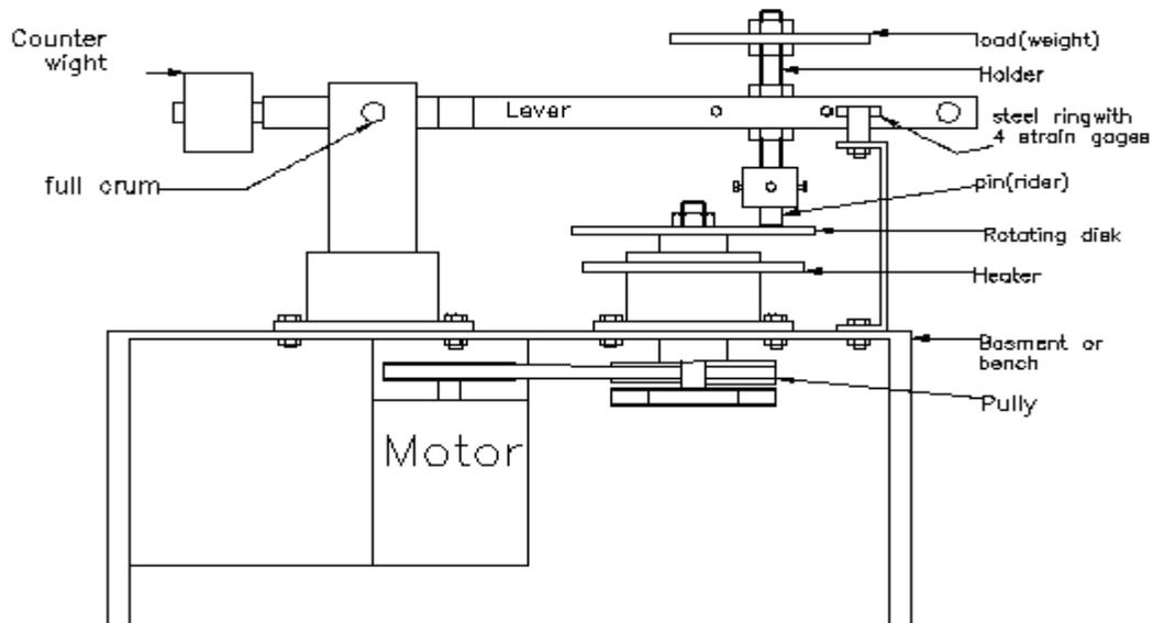
Figure 1. The Pin-On-Disc wear apparatus
