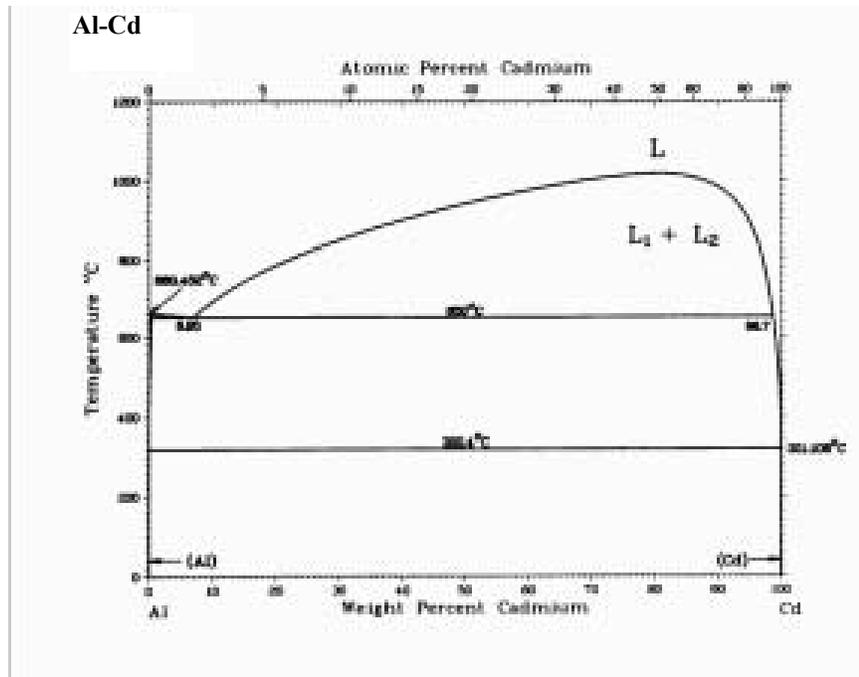
Figure 6. Phase diagram of Al-Cd alloys (Davis, J.R. and Associates, 1982)
