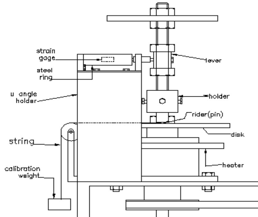
**Figure 2. Four strain gages mounted on steel ring in addition to strain gage calibration system**
