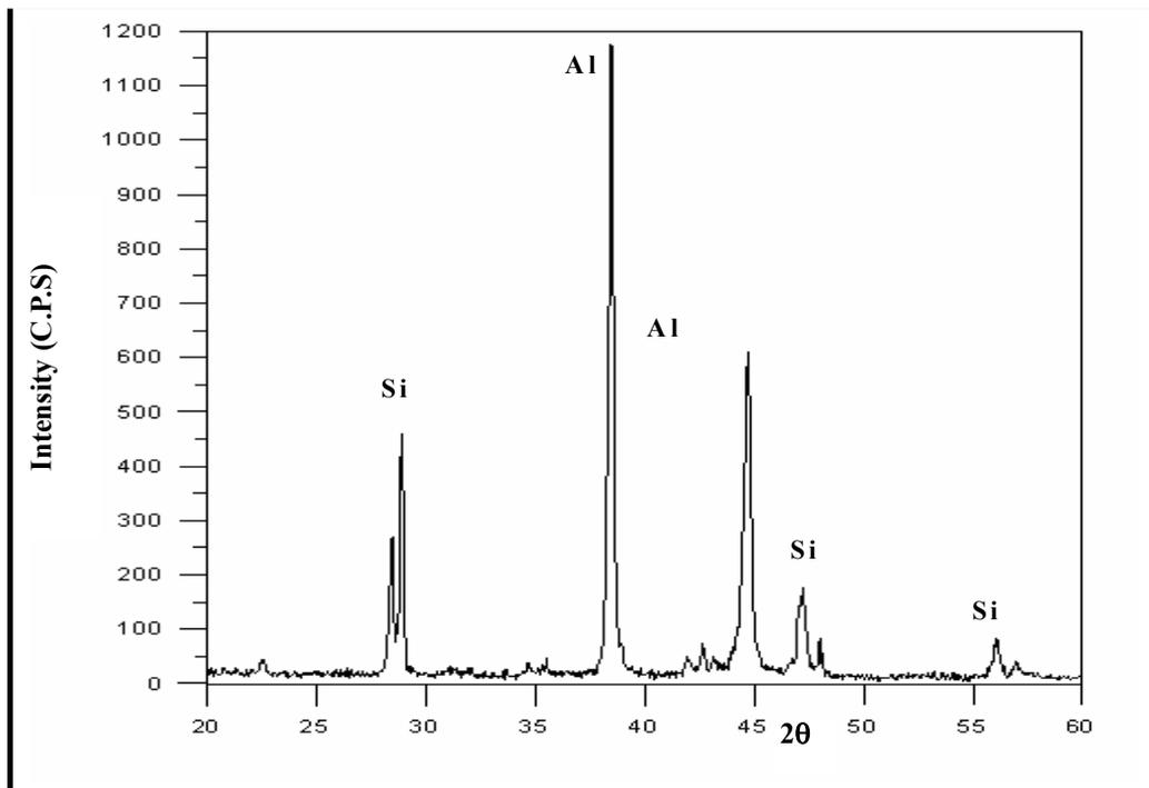
Figure 7. XRD results of an alloy (Al-12%Si - 3%Cd)
