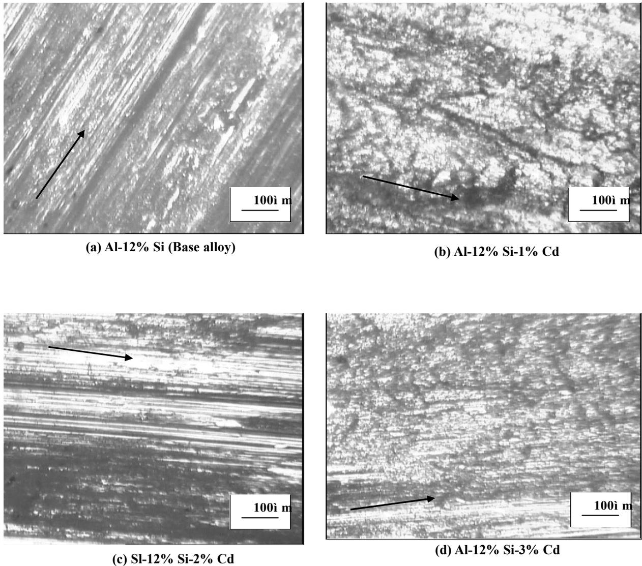
**Figure 10. Micrographs of the worn surfaces of different alloys at a applied load of 20 N, sliding speed of 2.7m/sec and steel disc hardness of 35HRc → sliding direction**
