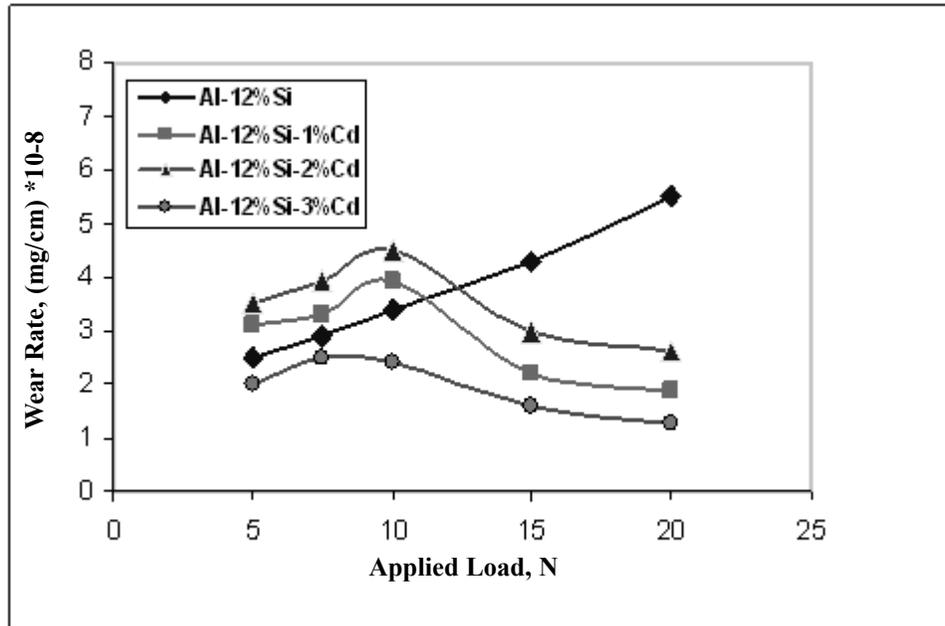
Figure 8. The effect of applied load on wear rate of different alloys at a sliding speed of 2.7 m/sec, sliding time of 20 min and steel disc hardness of 35 HRc
