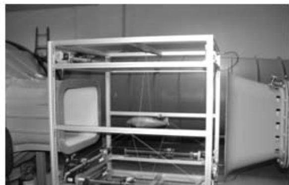
Figure 7. Wire-driven parallel suspension systems with 8 wires in the experiment of static derivatives.
