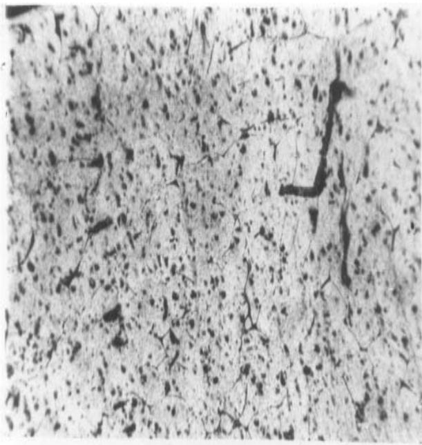
**Micrograph 2.** Microstructure of the Al-Si-Fe alloy with 10 wt% of SiC the the structure reveals the dissolution of the eutectic silicon phase and uniform distribution of SiC (black) in  $\alpha\text{-Al}$  matrix (white) (x200).
