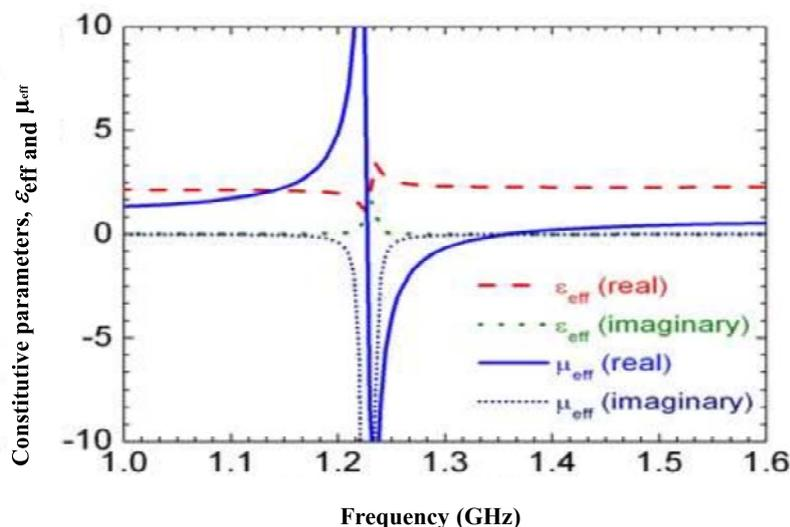
Figure 4. Effective response for the constitutive parameters of the SNG unit cell extracted using the retrieval method
