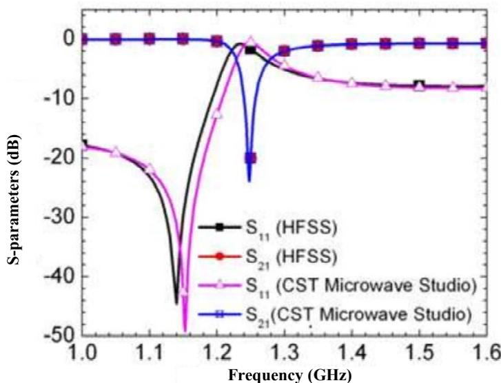
Figure 3. Scattering parameters of an SNG metamaterials' unit-cell extracted from the waveguide structure shown in Figure 2b
