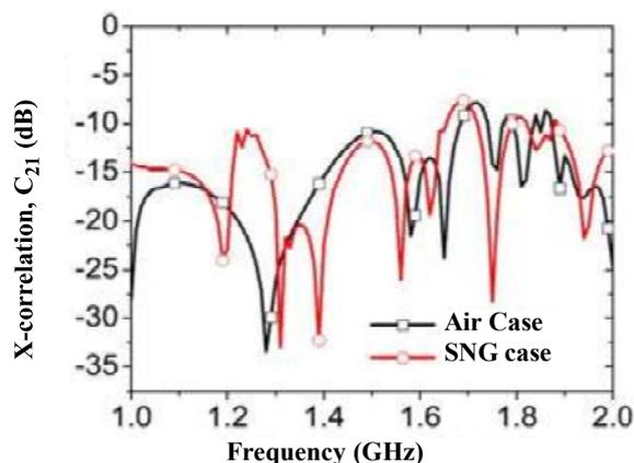
**Figure 13. Computed cross-correlation for the helical antenna system with and without SNG magnetic metamaterials**
