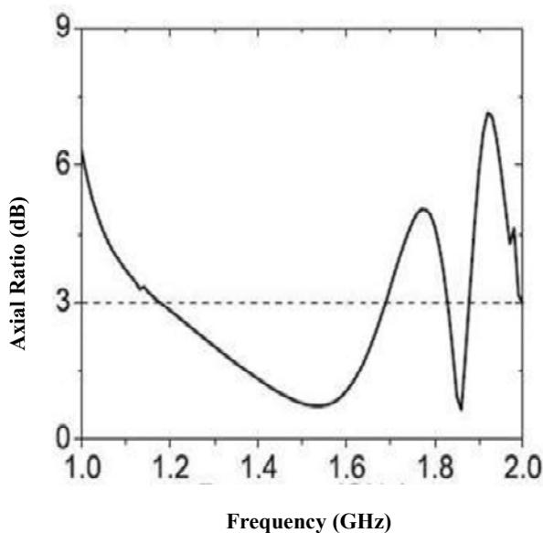
Figure 7. Frequency characteristics of axial-ratio in dB for the single helix antenna
