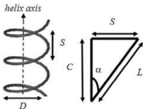
Figure 5. Design parameters of the helical antenna
