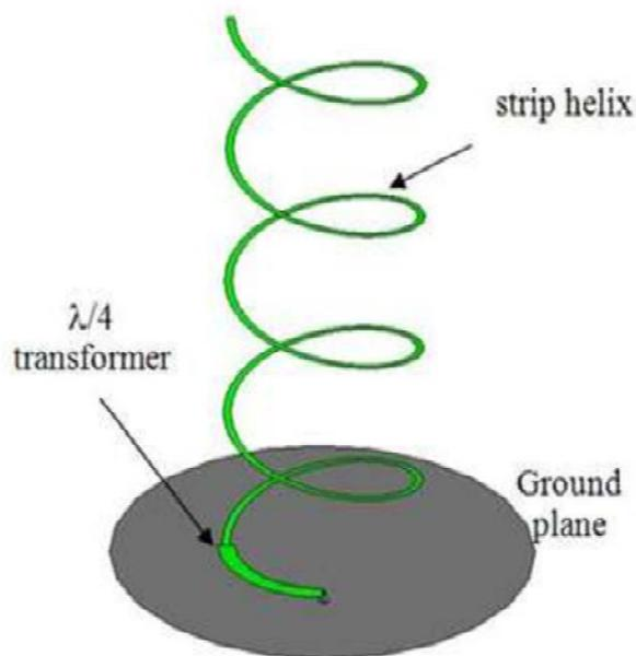
Figure 6. HFSS model for a single axial-mode helix antenna
