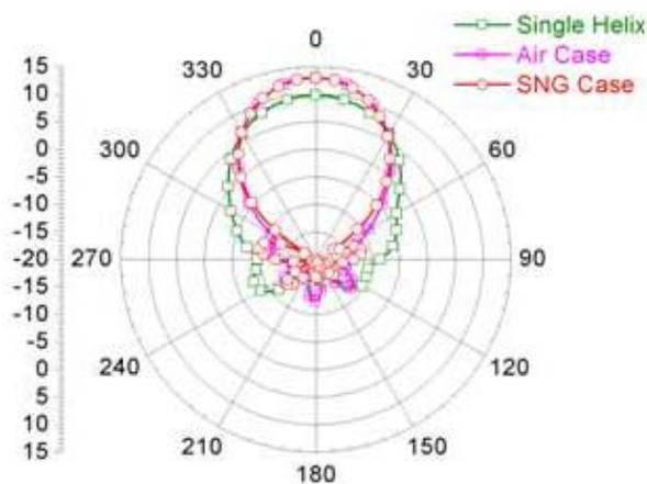
**Figure 14. Far-field gain pattern in axial-direction for the single-helix, the two helices with and without the magnetic inclusions, computed at a frequency of 13.1 GHz**
