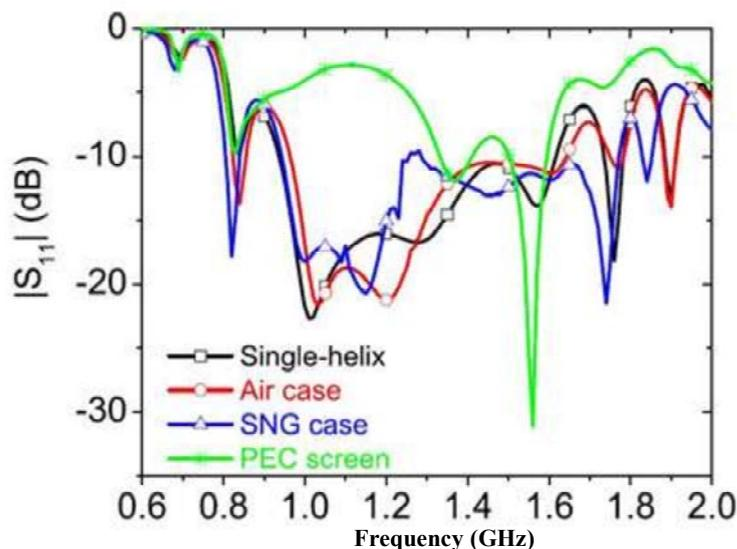
Figure 9. Magnitude of  $S_{11}$  for the helical antenna system with and without SNG metamaterials
