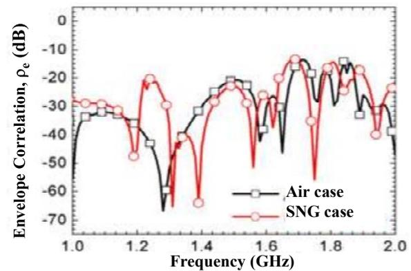
Figure 11. Envelope correlation,  $\rho_e$ , for the helical antenna system with and without SNG magnetic metamaterials
