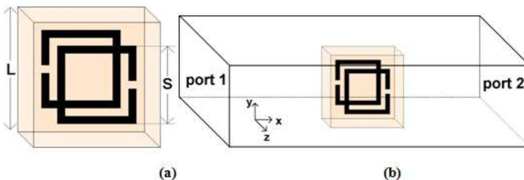
Figure 2. The developed single-negative magnetic metamaterials based on the (BC-SRRs): (a) Splitring resonator (SRR) unit cell with its dimensions, (b) waveguide structure used for the characterization of MNG metamaterials. Note the E-Field points in  $y$ -direction, H-field is in  $z$ -direction, and the propagation is  $x$ -direction
