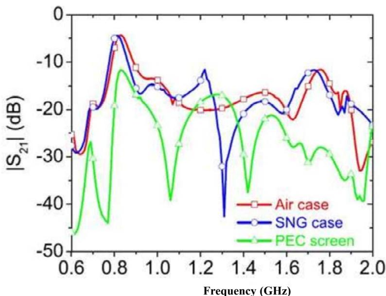
Figure 10. Magnitude of  $S_{21}$  for the helical antenna system with and without SNG metamaterials
