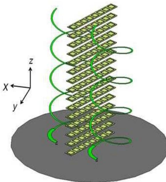
Figure 8. HFSS model for the two helical antennas with strips of single-negative metamaterials. Note that feed center-to-centre distance is  $\lambda_0/2$
