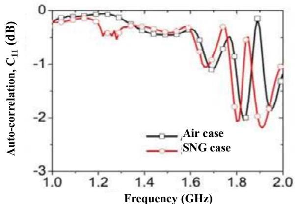
Figure 12. Computed auto-correlation for the helical antenna system with and without SNG magnetic metamaterials
