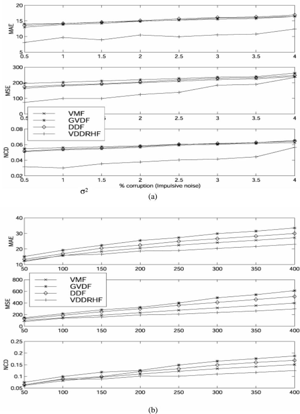
Figure 2. Comparative results for the color test images contaminated by Gaussian noise, (a) Pepper image, (b) Rose image
