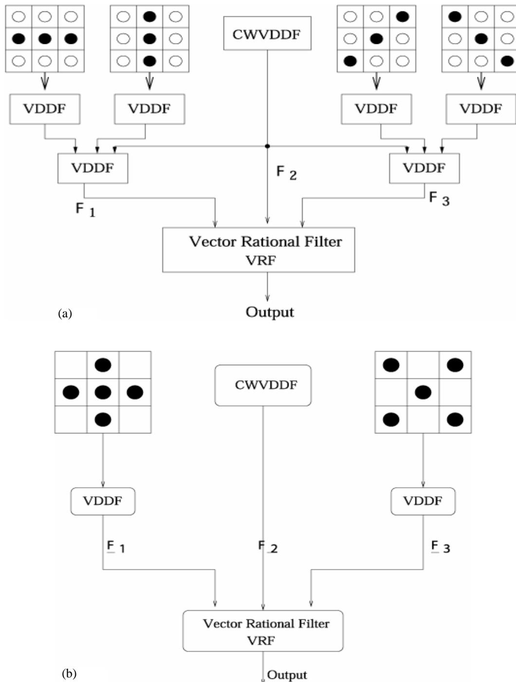
Figure 1. Structures of VDDRHF. (a) The unidirectional structure, (b) the bidirectional structure
