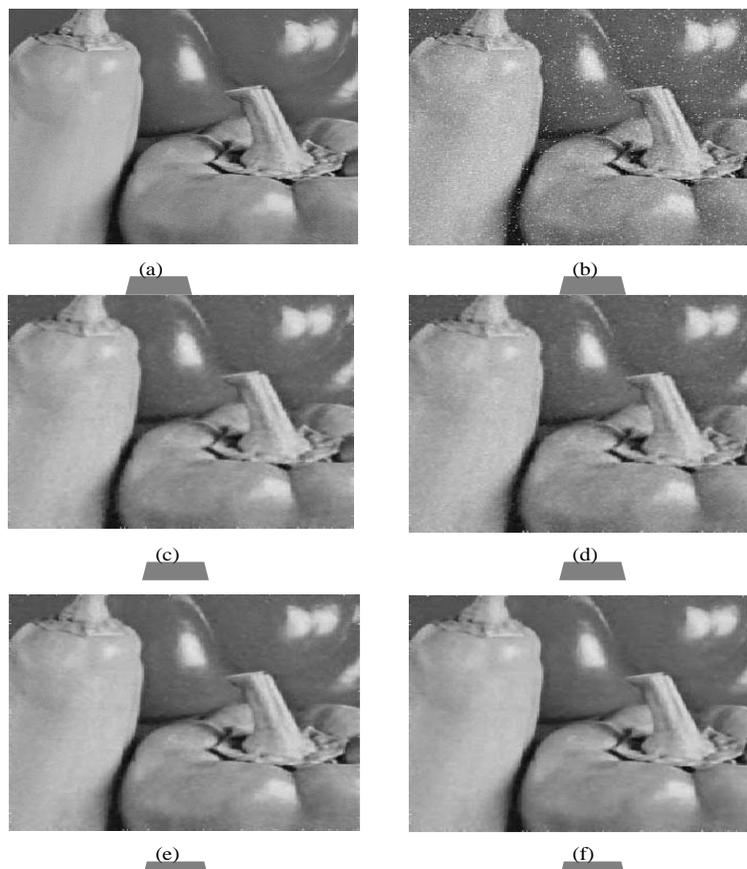
**Figure 6.** (a) and (b) are parts of the Original noise free and the contaminated Pepper image with additive (4% in each channel) impulsive noise, respectively. Images (c) - (f) are the results using DDF, GVDF, and VDDRHF, respectively
