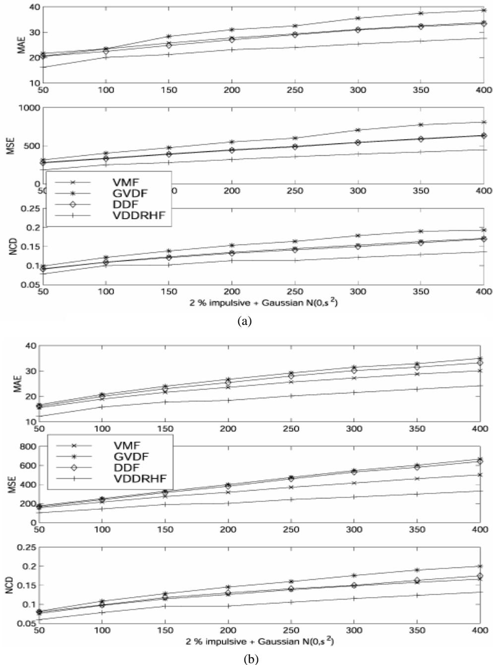
**Figure 4. Comparative results for the color test images contaminated by impulsive mixed noise (salt and pepper 2% in each component, and Gaussian with zero mean and variable variance), (a) Pepper image, (b) Rose image**
