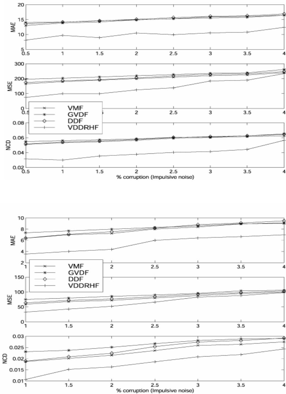
Figure 3. Comparative results for the color test images contaminated by impulsive noise (salt and papper). (a) Pepper Image (b) Rose image)
