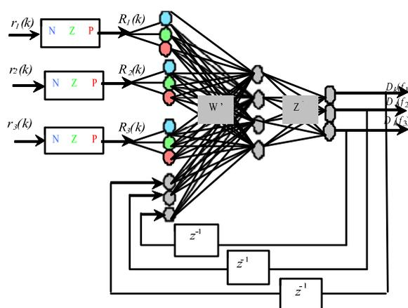
Figure 5. Example of a RNN used for residual evaluation
