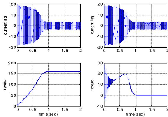
**Figure 6. Stator currents ( $I_{sd}$ ,  $I_{sq}$ ), rotor speed  $\Omega$ , torque  $T_e$  (normal operation)**
