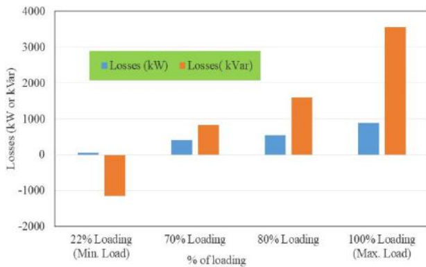
Figure 4. Total losses (kW and kVar) in the distribution network for different loading conditions.
